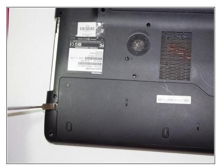
Using a spudger or plastic opening tool, pry off the service panel.
