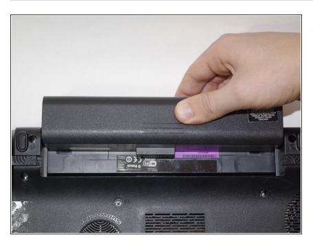
Pull the battery straight out of its slot to remove it.
