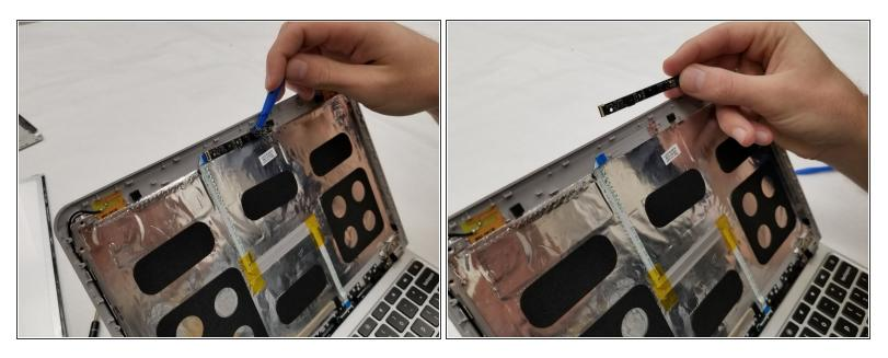
• Use an iFixit opening tool to pry the front camera assembly from the adhesive holding it in place.
