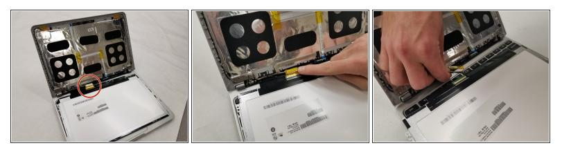
• Lift the lever to release the cable and pull the cable out.
