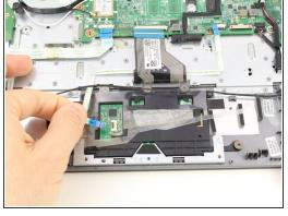
• Using a spudger, pry up the locking bar of the ZIF connector on the trackpad and remove the ribbon cable.
