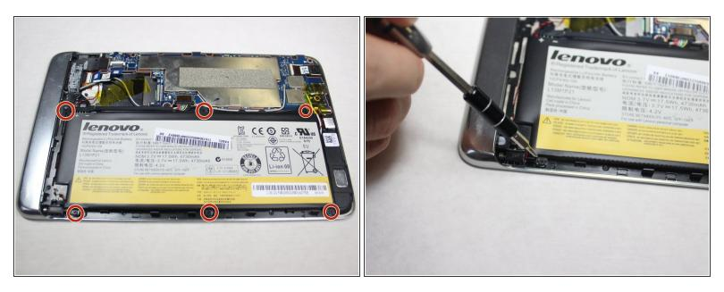
• Unscrew the six 3mm screws surrounding the battery dock using a Phillips #0 screwdriver.
