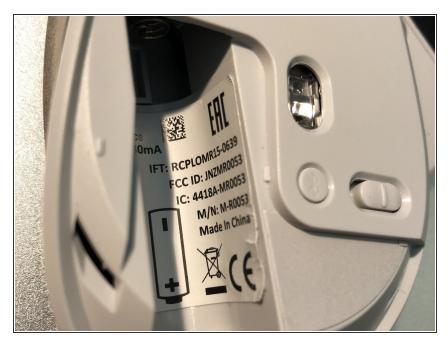
• Pull the sticker inside of the battery box slowly: the glue is pretty strong and the space is tight. A butter knife works alright. You need to remove enough of the sticker to get to the bottom of the battery box.
