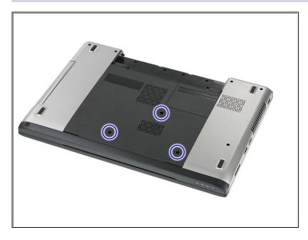
Remove the three 7mm Phillips #0 screws that secure the access panel to the base of the computer.
