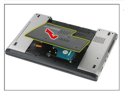
• Lift the access panel up at an angle and remove it from the computer.
