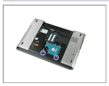
• Remove the two 5mm Phillips #0 screws that secure the hard drive to the system.
