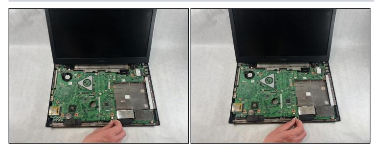
• Remove the small cable connecting the motherboard to the rest of the computer.
