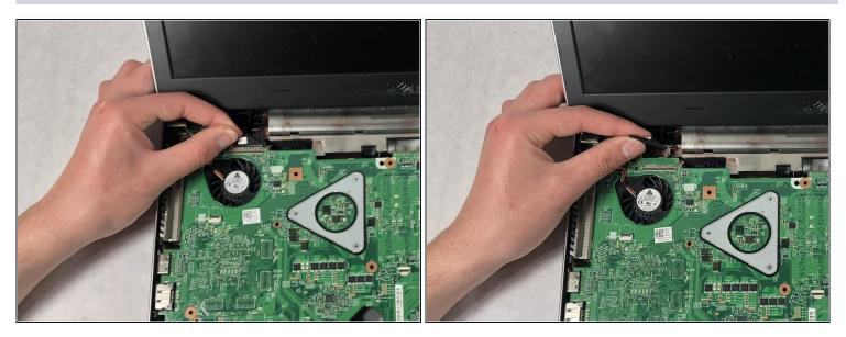
• Remove the ribbon cable at the far left that is connecting the motherboard to the screen.
