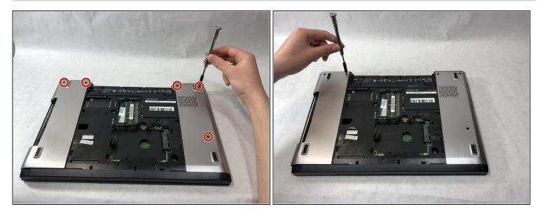
• Remove the five 7mm Phillips #0 screws fastening the aluminum side panels to the laptop.
