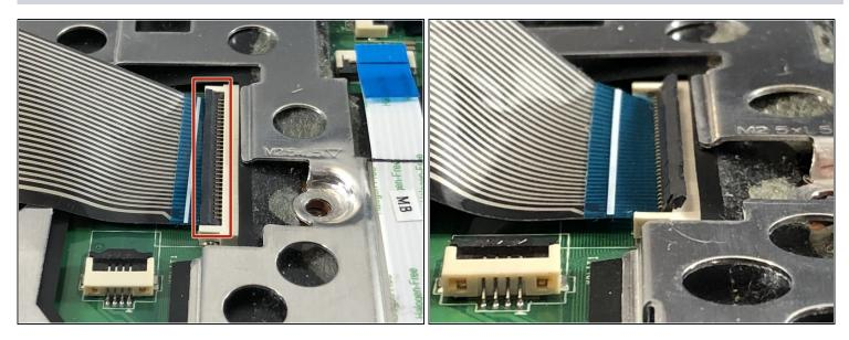
• Lift the black tab on the keyboard cable connector upwards to release the cable.
