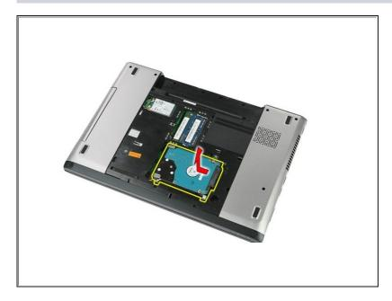
• Lift up the hard drive at an angle from the system and remove.
