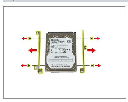
• Remove the four 5mm Phillips #0 screws that secure the hard drive bracket to the hard drive.
