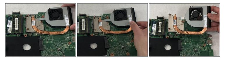
• Gently lift the fan assembly and heatsink away from the motherboard, and put it down onto a flat surface.
