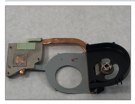
• Once the fan is removed, gently push the new one onto the motor.
