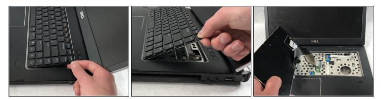
• Carefully lift the keyboard upward to reveal the keyboard ribbon cable.
