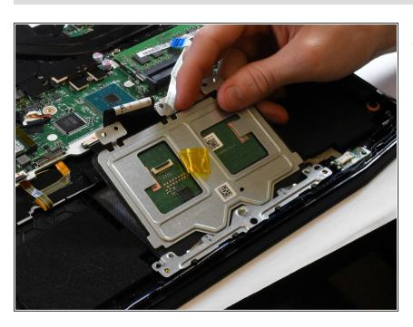
Lift up the Touchpad and remove it from the device.
