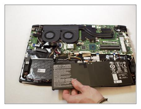
Remove battery from device.
