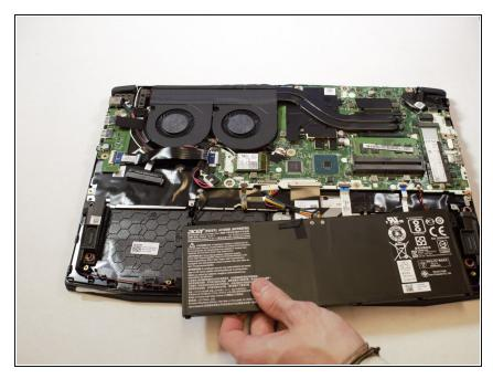
• Remove battery from device.
