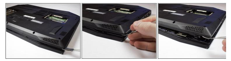
Be sure you removed the hard drive. when you open the back shell and hard drive is built in this may cause damage to cable and other components.
