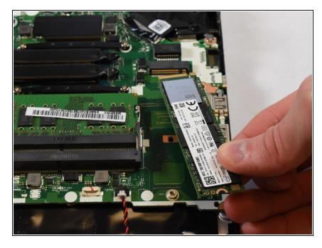
• Slide the SSD out of its slot.
