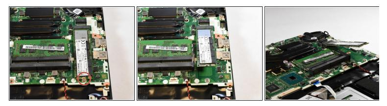
• Use the Phillips #0 screwdriver to remove the 3mm screw holding the SSD card in place.
