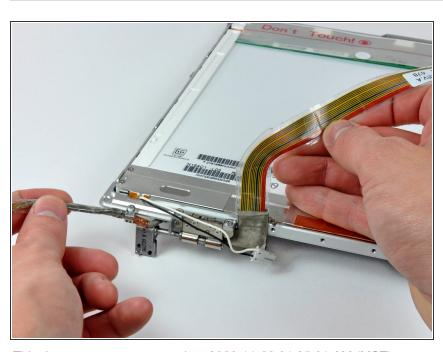
De-route the display data cable from around the right clutch hinge and remove it from the front bezel. To reassemble your device, follow these instructions in reverse order.
