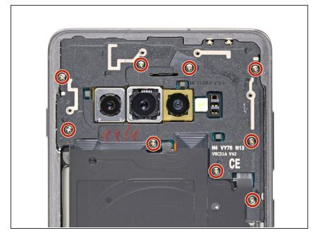
Remove the nine 4 mm Phillips screws securing the top midframe to the phone.
