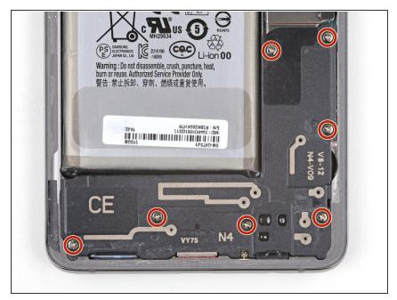
Remove the seven 4 mm Phillips screws securing the lower midframe to the phone.
