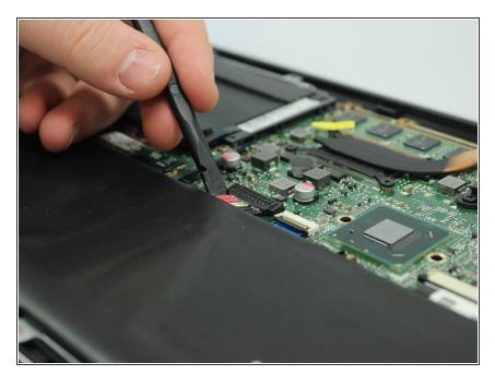
Disconnect the battery ribbon cable from the motherboard.
