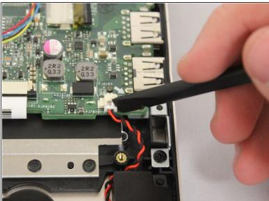
Unplug and remove the CMOS battery.
