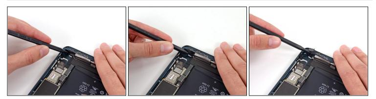
• With the tip of a spudger, peel up the larger piece of tape covering both antenna cables near the bottom of the rear case.
