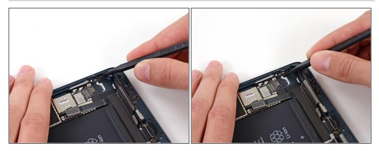
• Use the tip of a spudger to peel back the small piece of tape covering both antenna cables located near the bottom right corner of the iPad.
