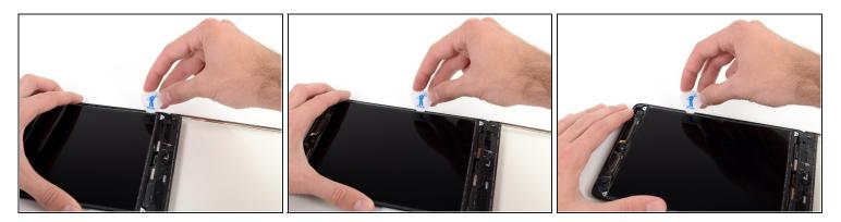
• Now switch to the right side of the LCD, and pry with the guitar pick in several places along the side to shift the LCD back to the left.
