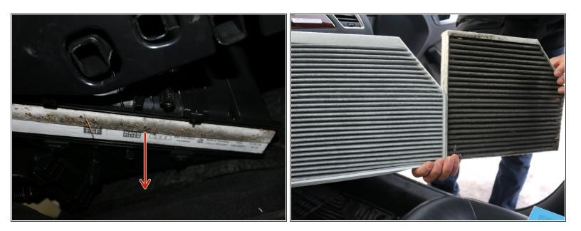
Pull the filter down to remove it.
