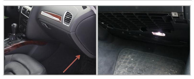
Locate the cabinet air filter under the passenger's glove box.
