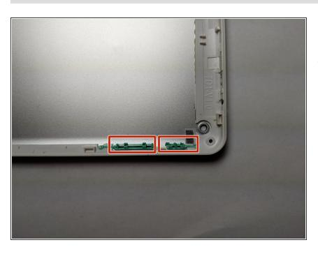
The power and volume buttons are on the side of the device. Locate these buttons to begin the replacement process.
