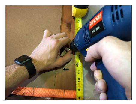
Use a power drill to screw in the screw and loop combo on both sides of the frame.
