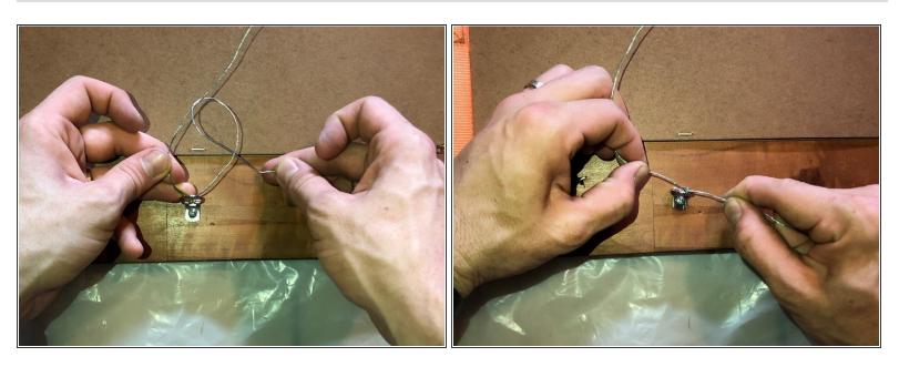
With the wire through the loop, tie like a regular knot and give it a good tug.
