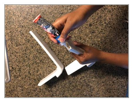
Spread the Loctite 60 Sec Universal glue along the edge of both sides of the bar.
