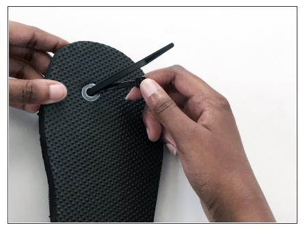
• Push the 4.8mm metal flat washer inside the hole of the flip-flop.
