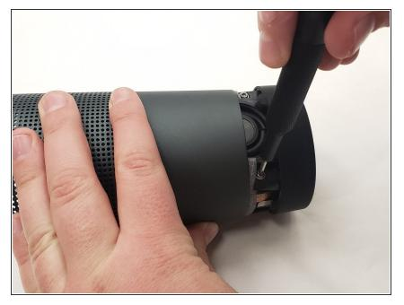
Use a T10 screwdriver to remove the four 6 mm screws around the 2 speakers, and remove the speaker units from the body.
