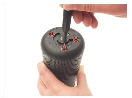
Use a T10 screwdriver to remove the three 10 mm screws from the bottom of the speaker.
