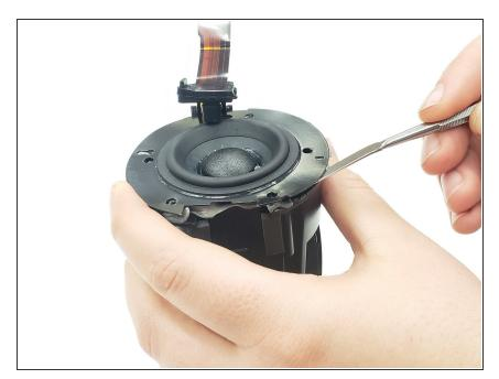
• Use a spudger to pry apart the glued section between the speaker panel and the device.
