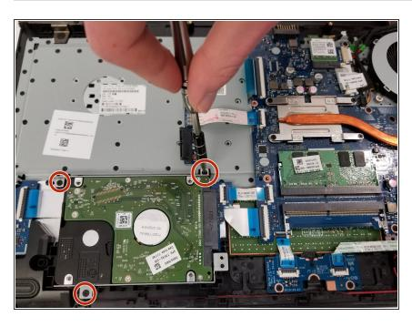
Remove the three 3 mm screws that mount the hard drive to the computer.
