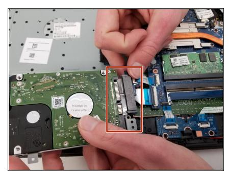
Remove the connector from the hard drive by pulling it away from the drive.
