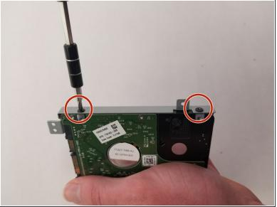
• Lift the hard drive from the computer and remove the two 3-mm screws that connect each mounting bracket to the hard drive.
