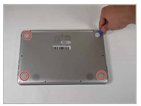
Use the iFixit opening tool to remove the 4 pads to reveal six 3.1 mm screws underneath.
