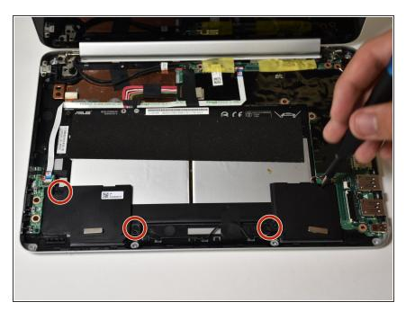
• Use the JIS1 screwdriver to remove the four 2.1 mm screws around the audio cards.
