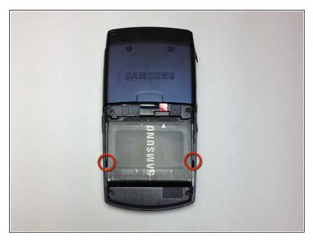
Use your fingers to pull the battery out of its position. You may also flip the phone and the battery will fall out.
