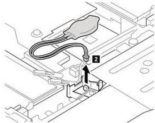
**When installing:** Make sure that the battery connector **2** is firmly attached.
