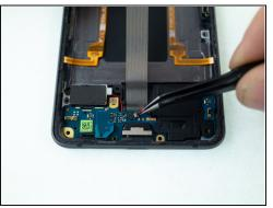
• Disconnect the speaker from the motherboard with a pair of tweezers.
