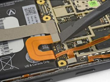
• Use the flat end of a spudger to disconnect the battery connector.
