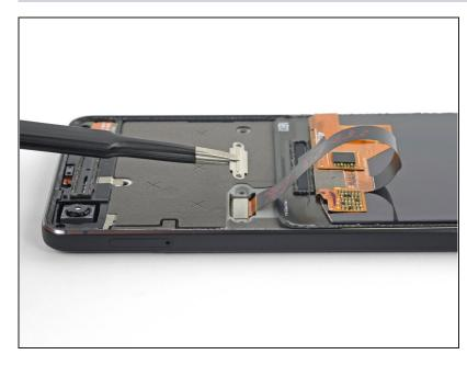
Remove the display cable bracket.
