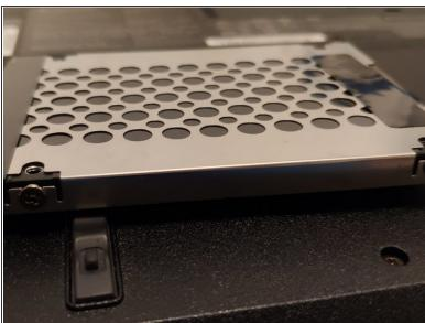
Remove the two rubber sleds from the drive caddy.
