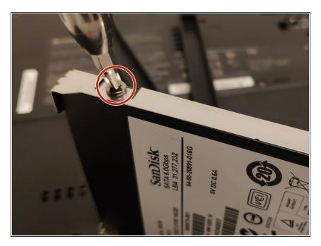
Remove the four phillips head screws around the hard drive. Do not lose these, as they will be used to install your new hard drive or SSD!
