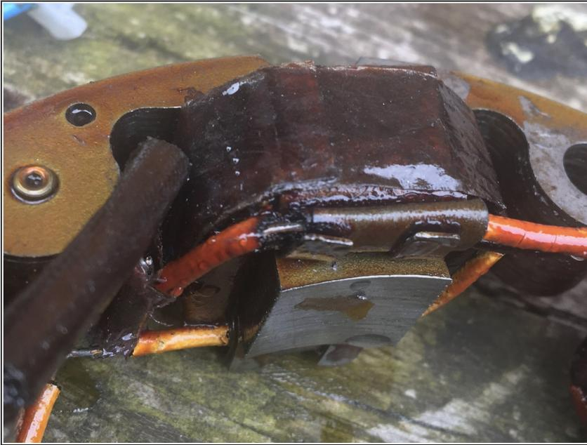
ⓘ The alternator stator is supposed to be insulated from earth.
