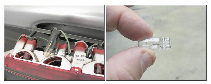
Remove the lamp socket and change the burned-out bulb (12V 5W).
