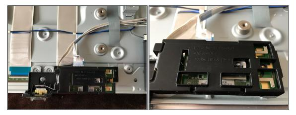
• To remove the Wi-Fi and Bluetooth module, there is only one screw holding the entirety of the structure.
