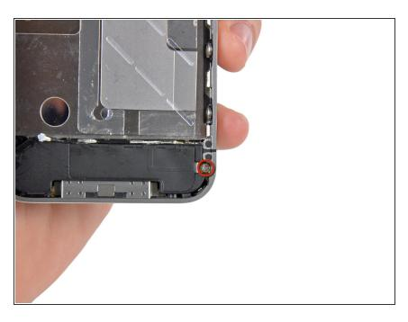
Remove the single 2.4 mm Phillips screw securing the speaker enclosure to the side of the inner frame.
