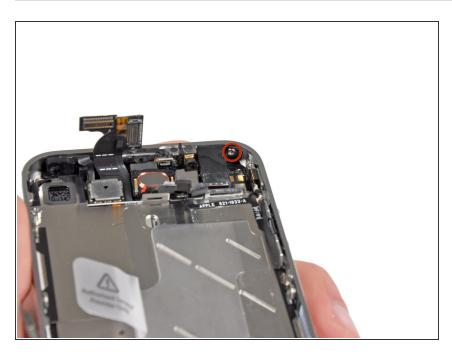
Remove the 1.5 mm Phillips screw securing the front panel near the headphone jack.
