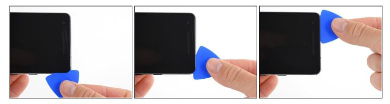
Slide the opening pick around the upper-right corner and along the top edge of the phone.
