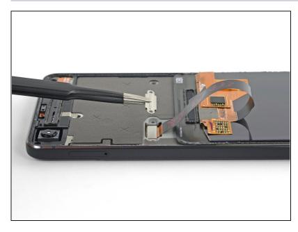
Remove the display cable bracket.
