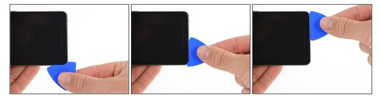
• Slide the pick around the bottom-left corner and along the bottom of the phone. Keep pick at a slight angle away from the screen to avoid damage to the OLED corners.
