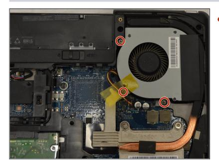
Once the back panel is removed and the fan is accessible, remove the three 3 mm screws holding the fan in place using a Phillips #00 screwdriver.
