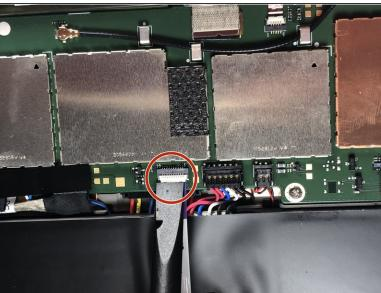
Remove the ribbon located over the battery.
