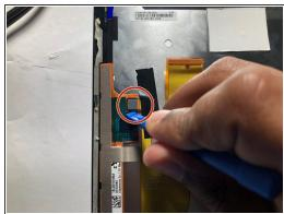
Use the plastic pry tool to remove both of the connections.
