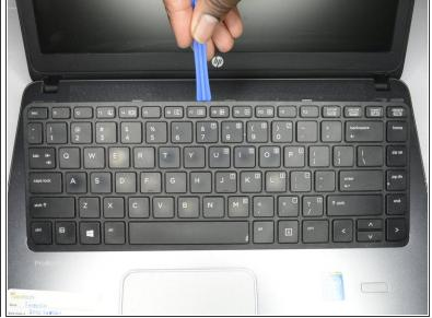
Using a plastic opening tool, pull the keyboard up.
