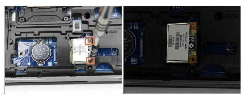
• Remove the two Phillips #00 screws holding the wifi card in place.
