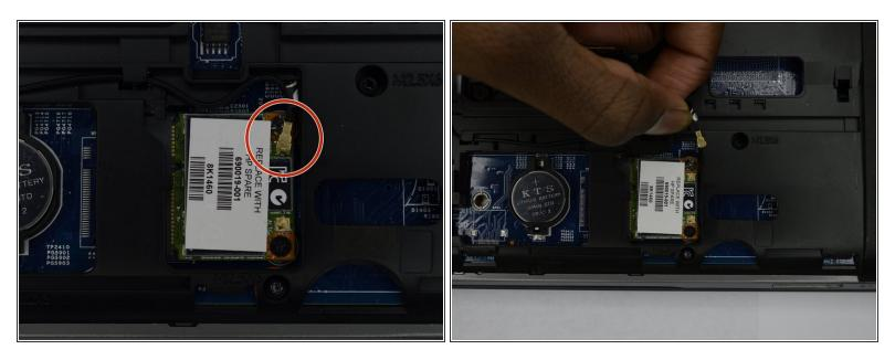
Remove the wire located near the screws on the wifi card.
