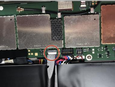
Remove the ribbon located over the battery.
