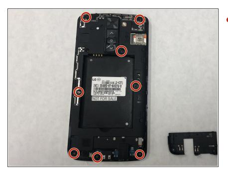
Remove eight 3mm screws using a Phillips #0 screwdriver.
