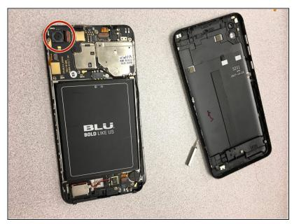
Identify the back-panel camera in the left -hand corner of the open device. (Figure 1)
