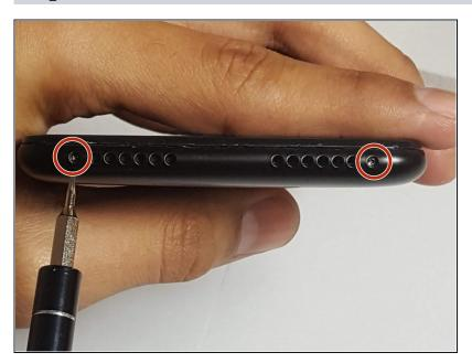
Locate the two torx screws at the bottom of the phone and remove them using the T2 Torx Screwdriver.
