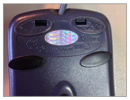
Using a spudger, release the clips securing the top of the mouse. One of mine proved very stubborn, so I needed to use a flat-blade screwdriver to release. Work carefully so as not to damage the plastic tabs.
