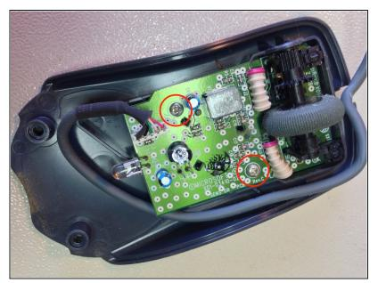
Using a Phillips #1 screwdriver, remove the two screws holding the lower PCB.
