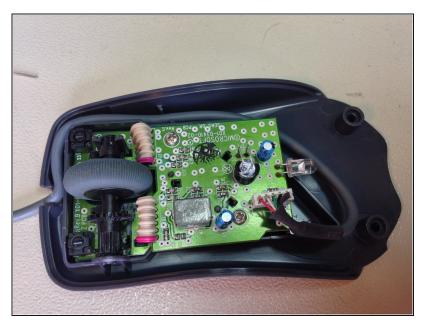
If there is any flux residue from soldering it may be cleaned with a little isopropyl alcohol. Now is an ideal time to clean out any dust and debris from inside of the casing before reassembly.
