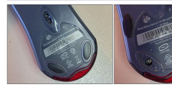
• Start by removing the four feet from the underside of the mouse. It may help to use a blade to lift a corner before gradually peeling off and setting aside.
