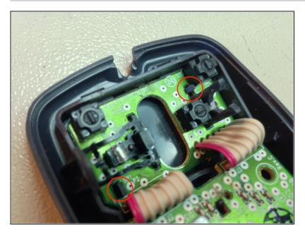
Remove the scrollwheel and release the upper PCB by depressing the two plastic tabs shown.
