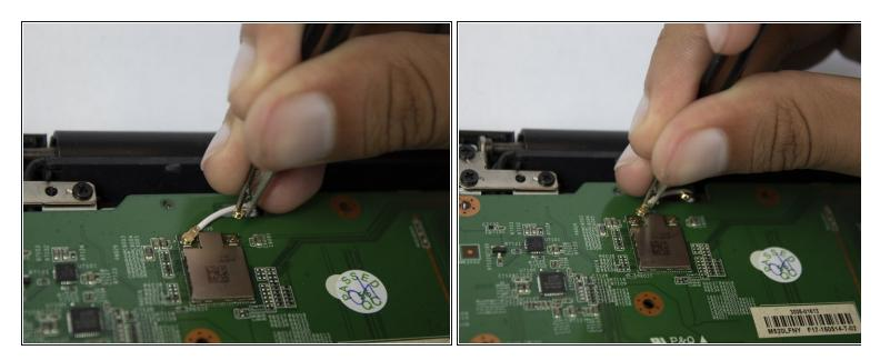
• Using the tweezers, carefully remove the latches attaching the silver computer chip.
