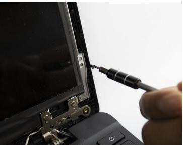
• Unscrew the screen screws with the Phillips #000 screwdriver and set them aside. Be sure to support the screen protector in case it falls.
