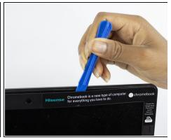
• Snap the plastic holds off of the screen protector using the plastic opening tool.
