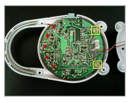
Remove the two screws securing the main board.
