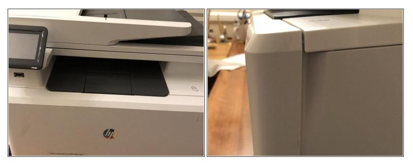
• find the two notches on the side that allow you to easily open the front panel.
