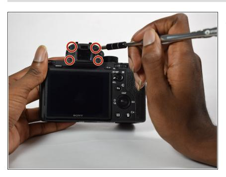
Remove the 4 screws on the viewfinder plate with a JIS #00 screwdriver.
