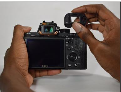
Carefully remove the plastic viewfinder plate from the camera.
