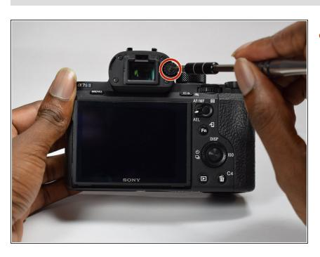
Remove the screw from the middle of the diopter with the JIS #00 screwdriver.
