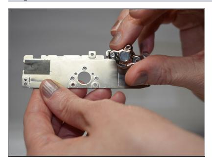
Remove the tripod mount from the metal plate.
