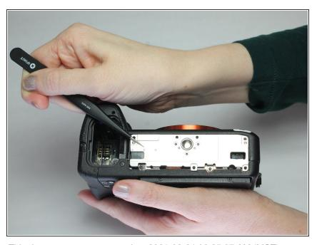
Remove the metal plate. Sometimes this plate can become stuck and hard to remove. Use tweezers to separate the plate from the bottom of the camera.
