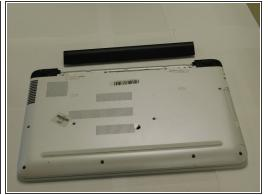
Slide the tab marked with a lock/unlock symbol. The slide the other tab in order to release the battery.
