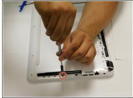
Remove all 16 size 3.5 mm screws with a PH1 screwdriver and pry the CD drive in order reveal one last screw that must be removed.
