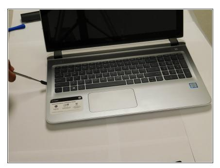
Utilizing either a plastic or metal opening tool, begin prying the case from the laptop. Lastly, remove the remaining clips located on the back of the laptop.
