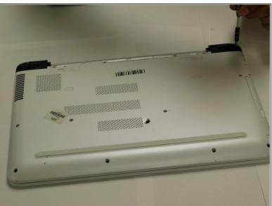
Once the battery is removed, unscrew and remove the both of the 7.5 mm screws off the black tabs using a PH1 screw driver. Then pry off the covers using the plastic opening tools.
