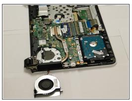
Utilizing a PH00 Screwdriver remove the two 3.5 mm screws detaining the cooling fan. Then use tweezers to remove the plug connecting the cooling fan to the mother board. Lastly remove the cooling fan.
