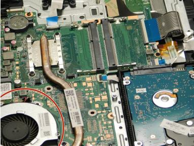
Once the laptop is fully open locate the cooling fan.
