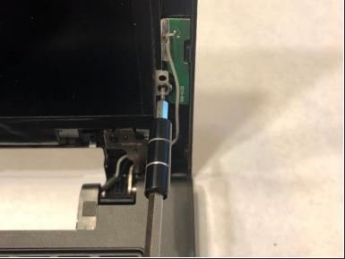
Unscrew four M2 x 3mm screws using a Phillips #000 screwdriver.
