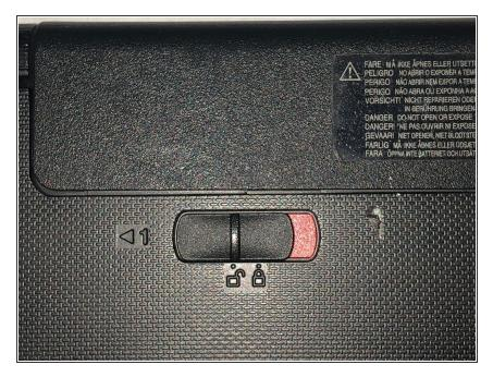
Slide the manual battery latch to the unlock position, so that the red is showing.
