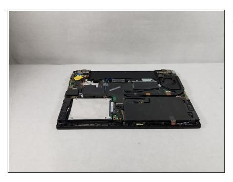
Remove the back panel from the device.
