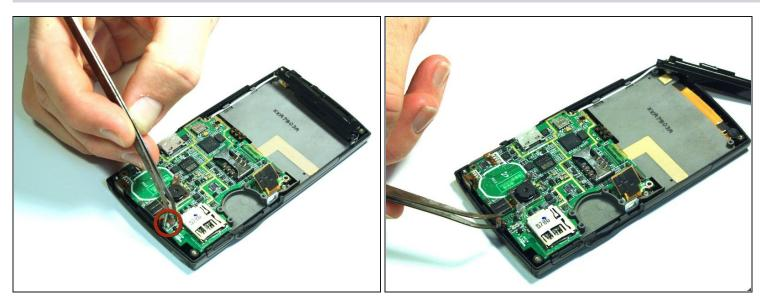
• Use the <u>tweezers</u> to unsnap the connection between the motherboard and the speaker. The speaker is attached to the front casing.
