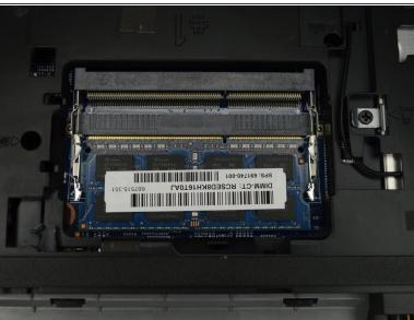
Locate the RAM, in the middle of the laptop near the battery.
